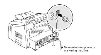
UK users should plug the cord of the extension phone into the supplied TAM lead and plug the cord of the TAM lead into the **EXT** jack on the back of your machine.
